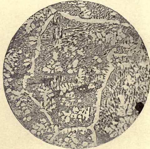
Fig. 35b. \times 210 Alloy 48. Cu 66.0 Slowly cooled in Sn 17.0 furnace. Zn 17.0. \gamma segregate + eutectoid.
